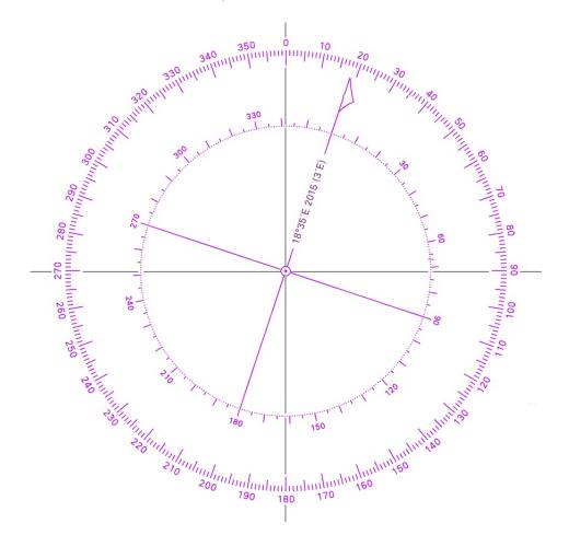
On a compass rose the outer circle shows True Bearings – the '0' at the top always points to True North.
